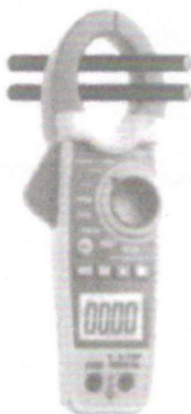
Incorrect Current Measurement
